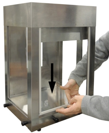
Lower Glass into Bottom channel
