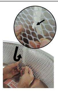
**Step 3:** Gently pull screening down and attach to bottom, down facing hook.
