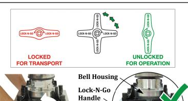
**Step 2:** Lock-N-Go® handles are used for transport. Rotate both handles to a vertical, UNLOCKED, position for use. This allows the bell housing to "float" freely on the springs during operation. **DO NOT operate with handles in the transport position.**
